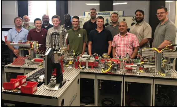
Figure 2 Mechatronics training lab (picture with transitioning soldiers from Fort Drum). This equipment has been complemented by customized PLC training elements.
