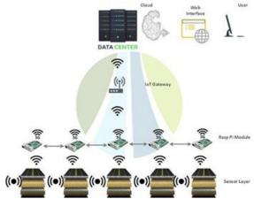
asphalt data will help to improve the quality of the asphalt with new findings by using this intensive data set and well know machine learning/modeling methods. Meanwhile, a low-cost solution, a customized multi-layered strain sensor, is provided to overcome the challenge (high temperature, high pressure) in asphalt pavement installation.
